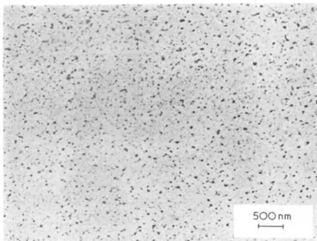
Figure 2 Electron micrograph of semi-IPN containing 30% by weight of polyurethane (sample E)
