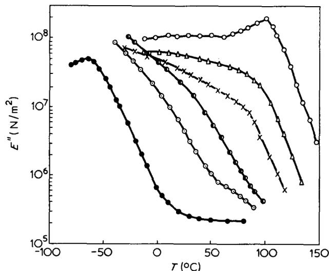
Figure 9 Dynamic loss modulus ( $E''$ ) versus temperature curves for polyurethane (●), modified polyester (○) and the semi-IPN's containing 70% (○), 60% (●), 50% (X) and 30% (△) polyurethane by weight
