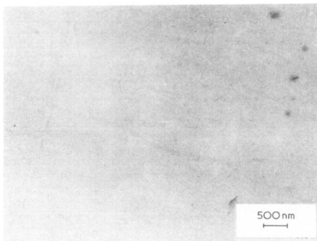
Figure 1 Electron micrograph of methyl acrylate modified crosslinked polyester resin
