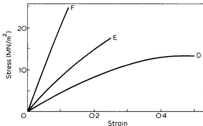
Figure 5 Stress-strain curves for the semi-IPN's containing 50% (D) and 30% (E) by weight of polyurethane and for the modified polyester resin (F)
