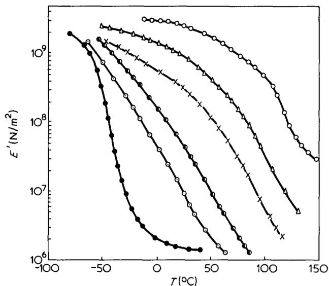
Figure 8 Dynamic storage modulus ( $E'$ ) versus temperature curves for polyurethane (●), modified polyester (○) and the semi-IPN's containing 70% (○), 60% (●), 50% (X) and 30% (△) polyurethane by weight
