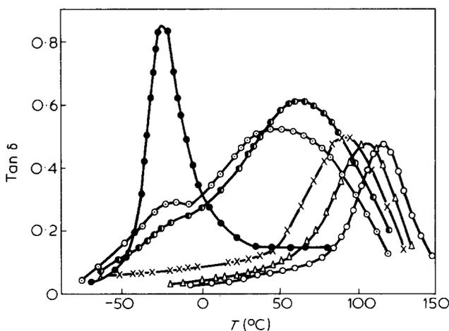
Figure 7  $\tan \delta$  versus temperature curves for polyurethane (●), modified polyester (○) and the semi-IPN's containing 70% (◊), 60% (⊙), 50% (×) and 30% (△) polyurethane by weight
