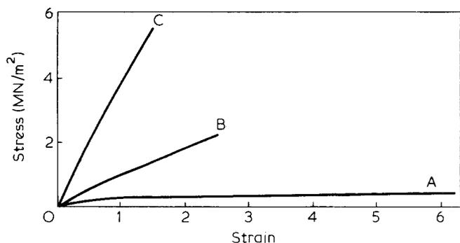
Figure 4 Stress-strain curves for linear polyurethane (A) and the semi-IPNs containing 70% (B) and 60% (C) by weight of polyurethane, respectively
