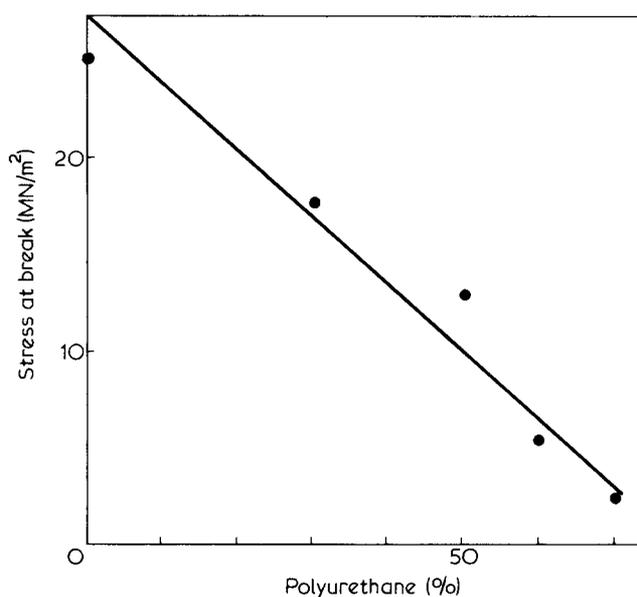
Figure 6 Curve showing stress at break versus weight % of polyurethane
