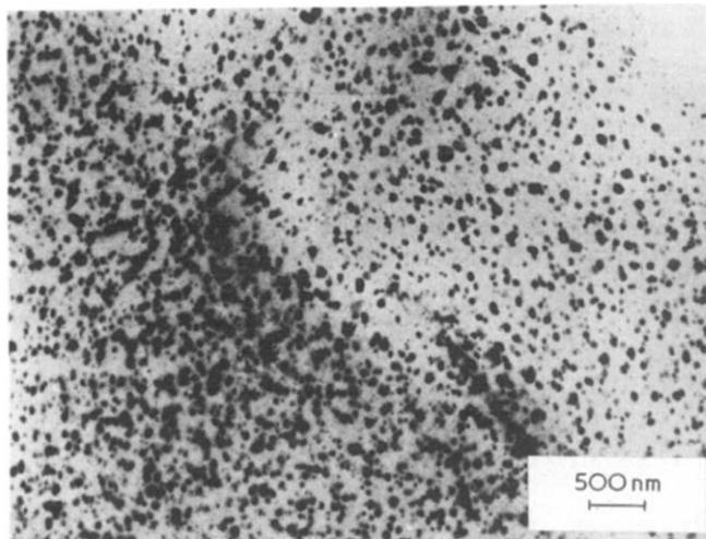
Figure 3 Electron micrograph of semi-IPN containing 60% by weight of polyurethane (sample C)
